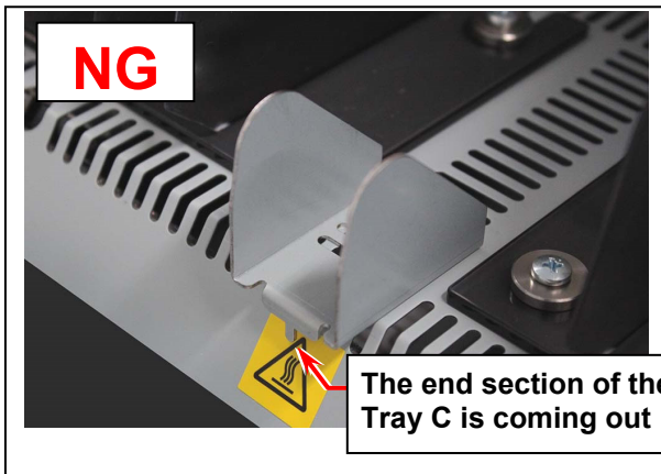
Incorrect : Inserted to the 4 th slit
