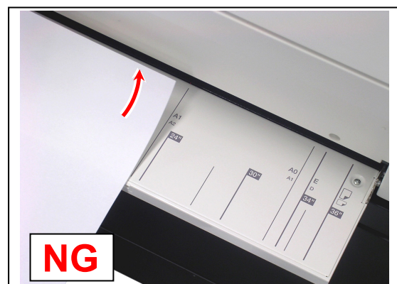
Incorrect (curl up)
